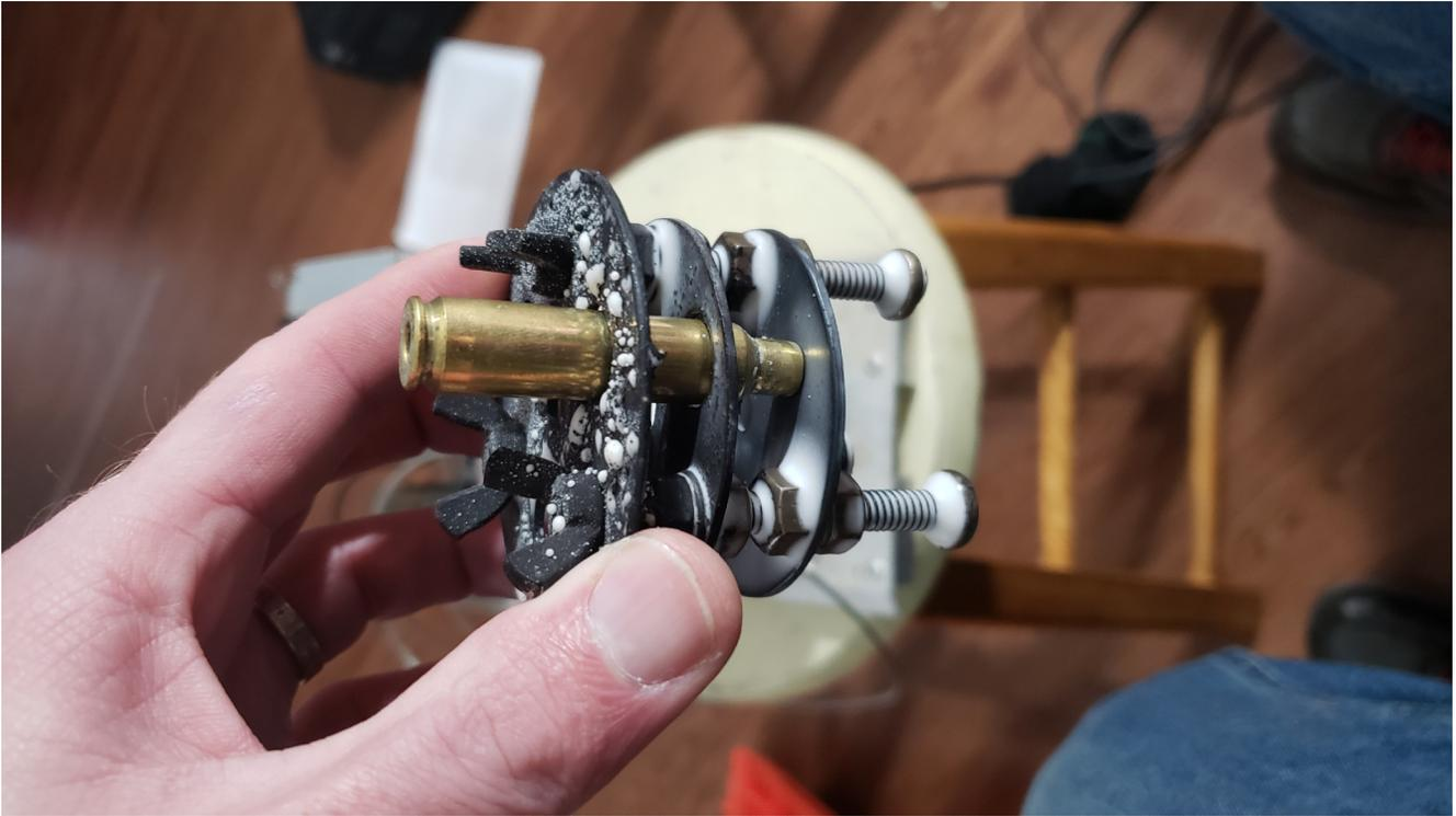
I keep the salt bath at the level of that middle plate (fender washer). This has holes for two cases and the temperature probe, but for the amount of shooting I get to do, one at a time is fast enough and much easier to keep straight. This is the one I use for 284Win, 7mm-08, etc. I also have one for 223 and 223AI.
