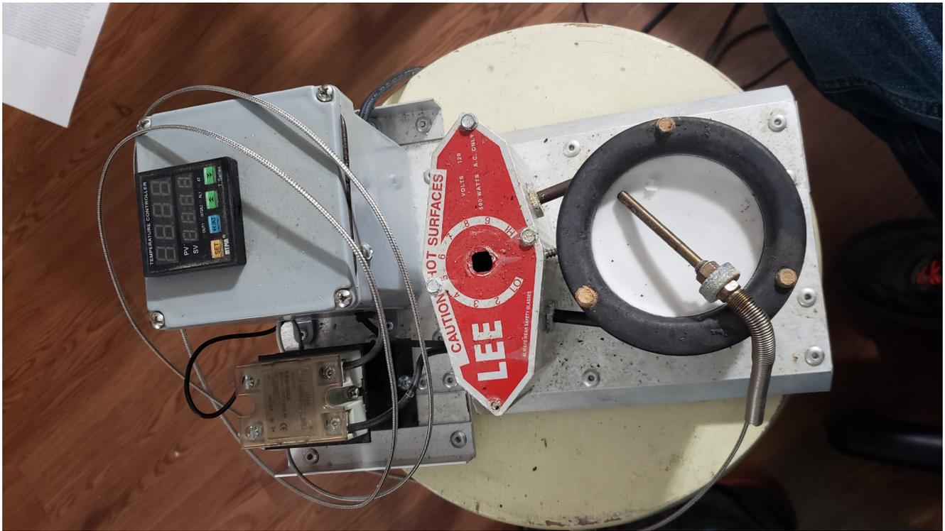
This is my salt bath annealer. The salt bath in the pot is pretty obvious, and the temperature probe (thermocouple) is sitting on the salt block. The PID is installed into the grey box (top left), which also houses a circuit block that I used to make hooking up the wires easier and avoid making soldered connections. The solid state relay (SSR, bottom left) sits on its heat sink, with the control wires on the left and the load circuit (power to the heating element) on the right.
