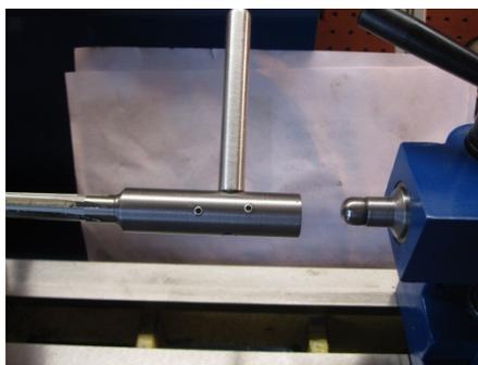
Place the barrel back into the spindle chuck and on tailstock center to indicate the barrel so that you have about 6 inches of barrel out. When the dial indicator is set up next to the screw chuck you can zero this short section of the barrel and it is very close to the bore line. Place and adjust the steady rest for chambering. This will leave about 8" for the chamber reamer and the floating reamer holder.
