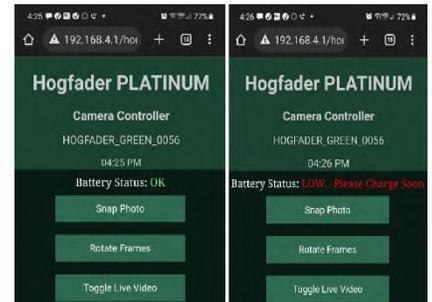
Note: It is very important to make sure that the antennae on the unit is oriented toward your location. This will provide the best signal. The 'Snap Photo' button will display a captured image from the camera on the screen and will save a copy of that image in .jpg format to the SD card inside the unit (the lid must be removed from the unit to retrieve the SD card). The 'Toggle Live Stream' button will display a live stream video of the action under the unit.
