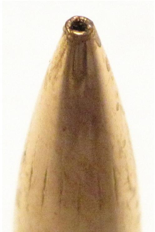
**Figure 6: Zooming in on a bullet's meplat reveals irregularities, which are normal and prevent consistent COAL measurements.**
