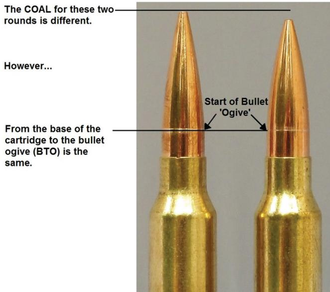
**Figure 4: Two different bullet shapes, seated to the same CBTO length, but different COAL. Note the shiny scratches on the bullets made by the comparator tool, which indicates a point on the bullet ogive near where the ogive will engage the riflings.**
