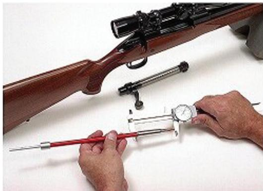
**Figure 5: Hornady 'Lock-n-load', formally known as the 'Stony Point Gauge'.**
