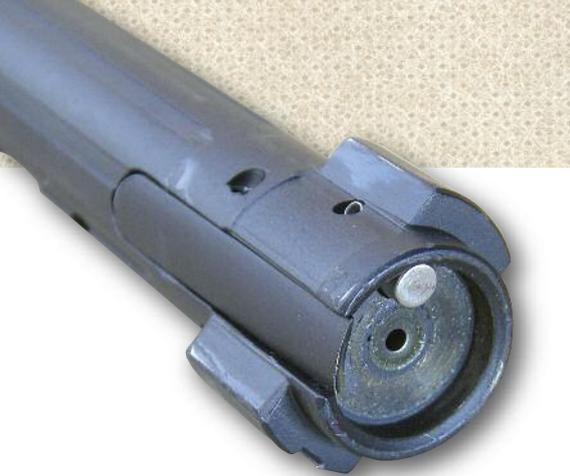
The twin-lug bolt head features a rotating extractor, plunger ejector and countersunk face.
