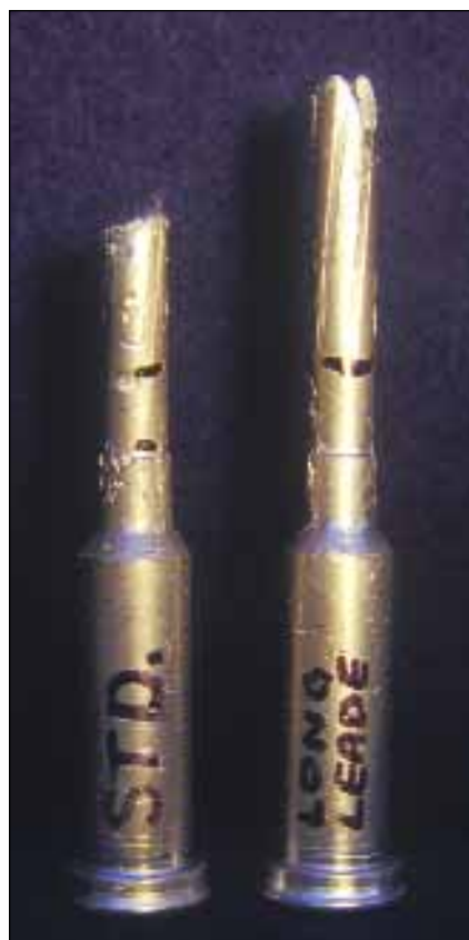
Left, chamber casts show the two different leades used in the test: factory SAAMI chamber and tapered leade (left) and factory chamber with modified straight leade to .250 inch (right). Below, the SAAMI chamber drawing.
