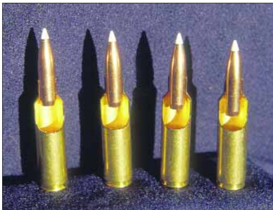
The .300 WSM cutaways show how far the bases of the bullets extend into the case at the four different OALs used in the test: (left to right) 3.000, 2.940, 2.880 and 2.820 inches.
