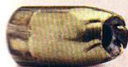
Fired Golden Saber™ bullet showing Driving Band contact area
