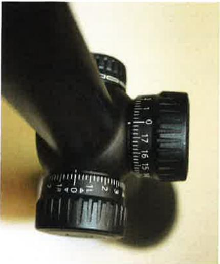
From the factory, the scope will have both the windage and elevation turrets set to "0".
