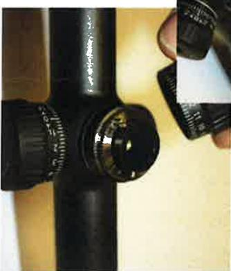
To re-set both the turret to the "0" reference as well as the stop mechanism, first remove the turret with a flat head screwdriver
