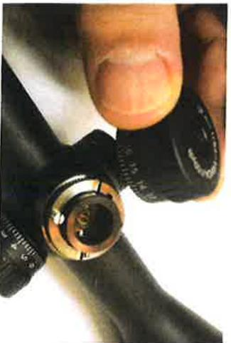
2. Lift the screw and turret cap off only. Leave the black collar inside the mechanism in place.
