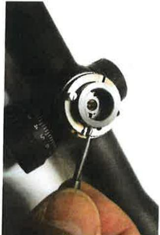
4. You can remove either or both of these to allow for complete use of the elevation (or windage) mechanism without stopping. Retain these for future use. (Note, the vertical pin is much easier to put back into place.
