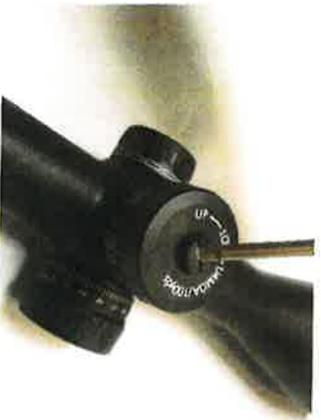
1. Remove the center screw that retains the elevation knob. (This process can also be used for the windage knob.)
