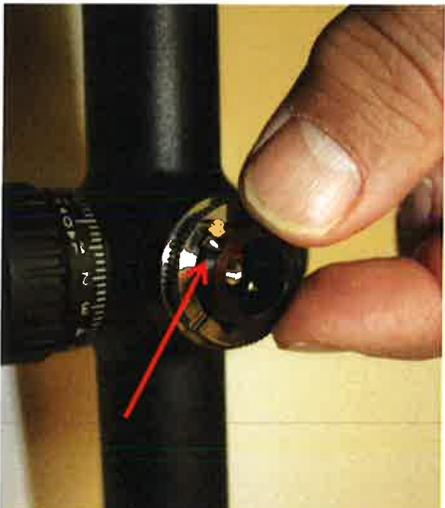
Place the black collar with pin back in the adjustment housing so the horizontal pin is right in front of the vertical pin – this is the correct position for the stop to work.
