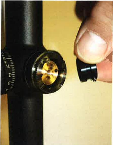
Once you remove the external numbered turret, you will see a black collar with a horizontal pin in it in the brass part of the adjustment mechanism. Remove this.
